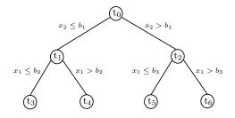
Fig 2: A maximal axis-aligned decision tree with depth K = 2 in p = 2 dimensions. Splits occur along individual covariates of the form  $x_i = b$  for j = 1, 2.
